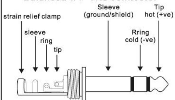
For connection of balanced and unbalanced plugs, ring and sleeve have to be bridged at the stereo plug.
