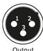
For unbalanced use, pin 1 and pin 3 have to be bridged
