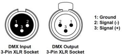
Caution at the unit, the DMX cable has to be terminated. Solder a 120 Ohm resistor between signal (-) and signal (+) into a 3-pin XLR connector and plug this into the DMX output of the last unit in the chain.
