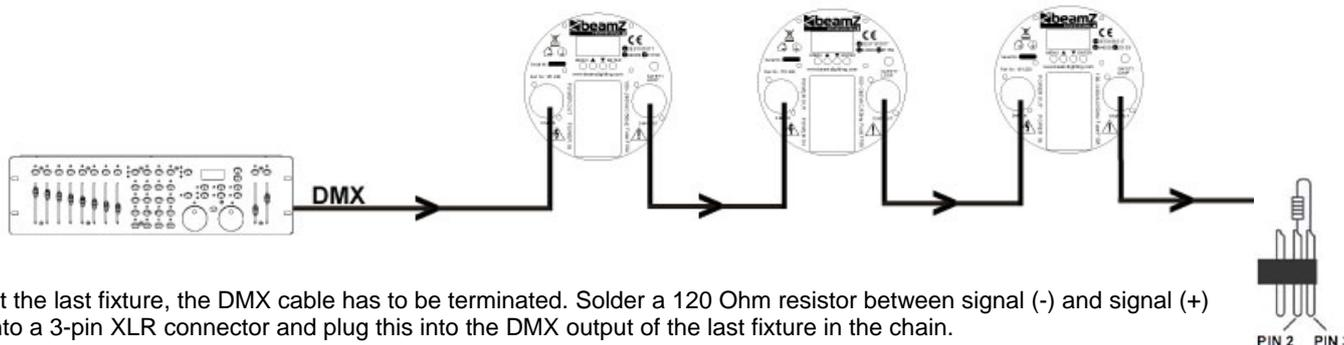
At the last fixture, the DMX cable has to be terminated. Solder a 120 Ohm resistor between signal (-) and signal (+) into a 3-pin XLR connector and plug this into the DMX output of the last fixture in the chain.
