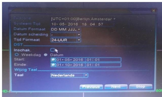
Then press "Next" to continue. Set the time and date correctly, here you can also set the summer and winter time. To activate this select Select DST, then enter the correct date and time. Then press "Next" when you have a router connected to an UTP cable, and you can see one of these images.
