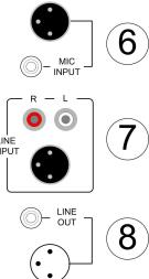
6. Balanced input connector CH-1 (XLR or 6.3mm Jack)
