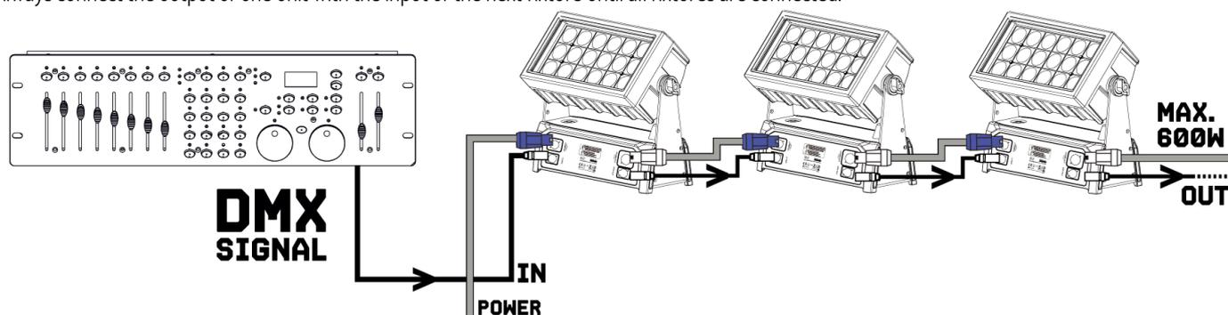
**Caution:** At the last fixture, you must close the DMX line with a terminating resistor. Take an XLR connector and solder a 120 Ohm resistor between signal (-) and signal (+) and connect it to the DMX output of the last fixture in the line.
